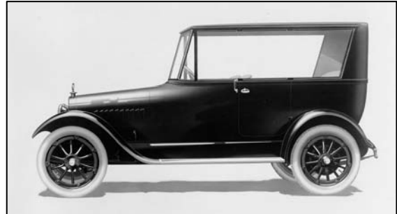
1917 Model 35-B Lucile Sedan with door & window posts removed
