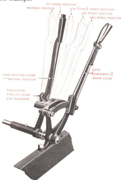
Fig. 14—Movements of Gear Shift Lever in Changing Speeds
