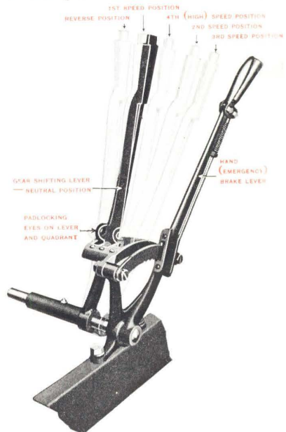
Fig. 14—Movements of Gear Shifting Lever in Changing Speeds
