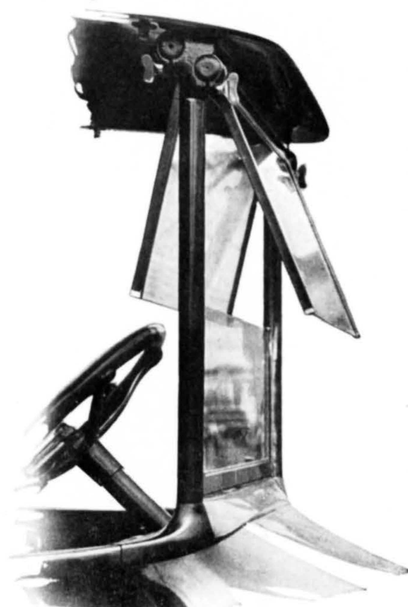
The windshield of the 1915 Chalmers Limousine is provided with double glass in the upper half, giving a positive clear vision even in heaviest rain or snow.
