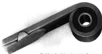
Rubber bushing in eye of rear spring absorbs road shocks
