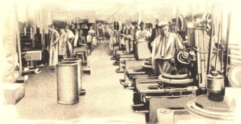
On these automatic gear cutting machines are cut all of the transmission, cam shaft, steering and pump gears which are used in Chalmers cars. No cars have higher grade, more accurately cut or more silent gears than those in the Chalmers.
